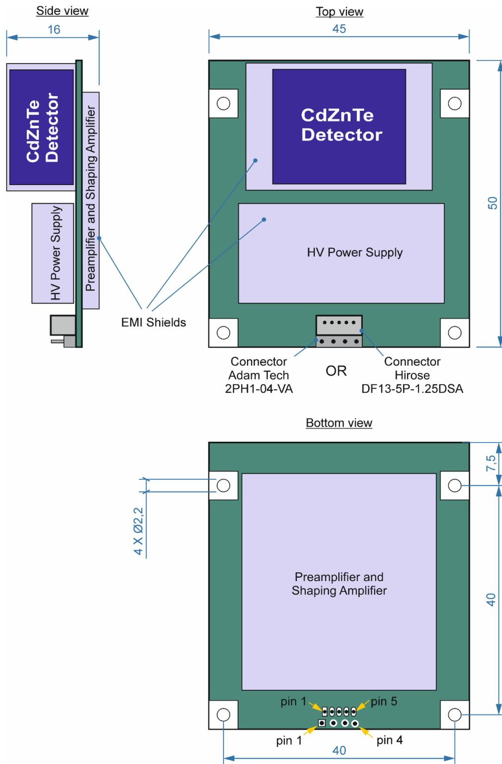
Fig. 4. Dimensions of the DM118 / DM118/L.
