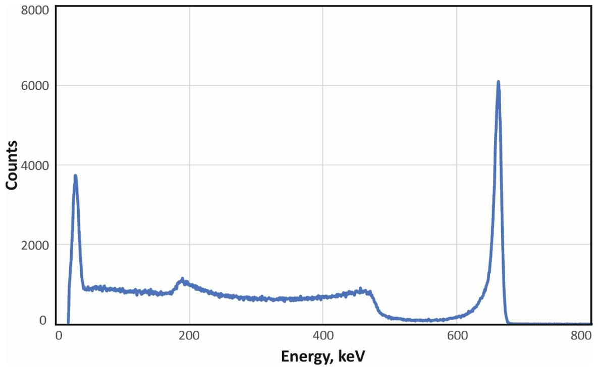
Fig. 2. Spectrum of  $^{137}\text{Cs}$  obtained with the DM118/L.
