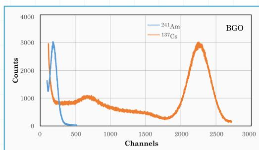
Properties of fabricated scintillator detectors measured at room temperature 20 °C under the same conditions
